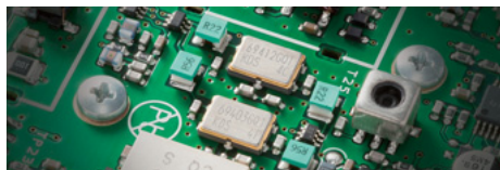
3 kHz and 15 kHz Roofing Filter
